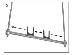
Slide TouchDown clamps to desired location within the bracket.
