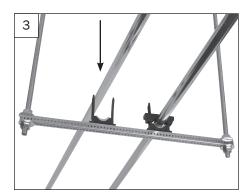
Position tube or conduit into base of TouchDown clamp.
